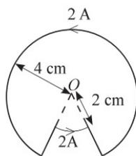
$$B_0 = \left[ \frac{\mu_0 I}{2 \times 4 \times 10^{-2}} \times 2\pi \times \frac{3}{4} \right] + \left[ \frac{\mu_0 I}{2 \times 2 \times 10^{-2}} \times 2\pi \times \frac{1}{4} \right]$$
